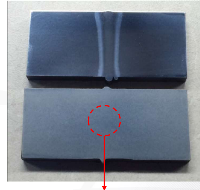
WCLs of EBW prior to and following HT
