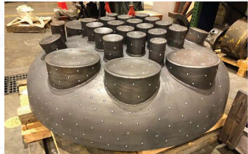
SMR vessel head (44% scale); A508/Gr. 3/Class 1 low-alloy steel powder (1,650 kg). 27 penetrations
